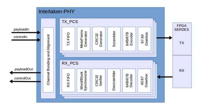
The sFPDP-Gen3 Framing Layer implements the 64B/67B Framing Layer defined by the Interlaken v1.3 specification. The Framing Layer supports single-lane and multi-lane channel bonding with automatic link synchronization. A per-lane CRC32 is calculated in order to guarantee link integrity and assist with channel diagnostics. The Framing Layer exchanges data between the sFPDP Protocol Link layer and the FPGA transceiver(s).
